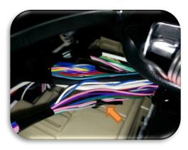
Tape the lead OBD socket remove to enlarge Available cable length.
