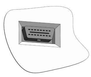
remove the original OBD socket jack from it's housing
