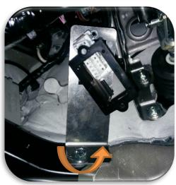
Bracket mount with just dissolved screw -- Lead OBD socket through the hole and add with the lower part of OBDS. Rotate bracket till the OBD-Socket/cable lengt fit
